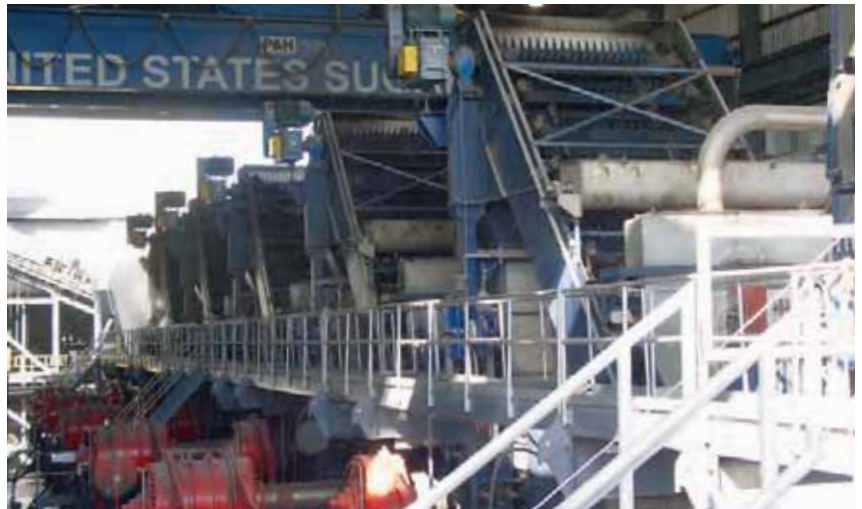
U.S. Sugar's new C Tandem mill replaced the nearby Bryant facility that was shut down. The new milling tandem was built with its own cane dump, cane preparation and conveying systems, with more than twice the capacity of the older B tandem.
